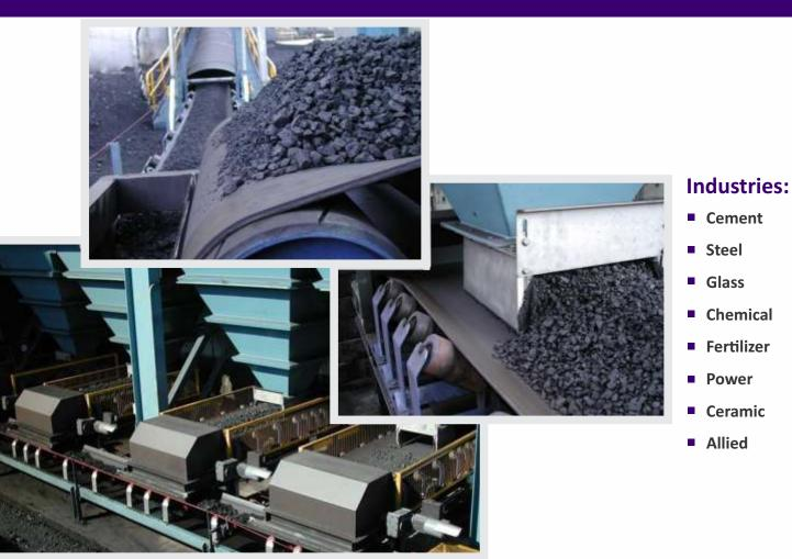
Enweigh Belt Weigh Feeders are designed for continuous heavy-duty environments either indoors or outdoors. The Weigh Feeders will accurately weigh any bulk solid material the conveyor will carry and will accurately control the flow rate of bulk material for product blending or process control.
